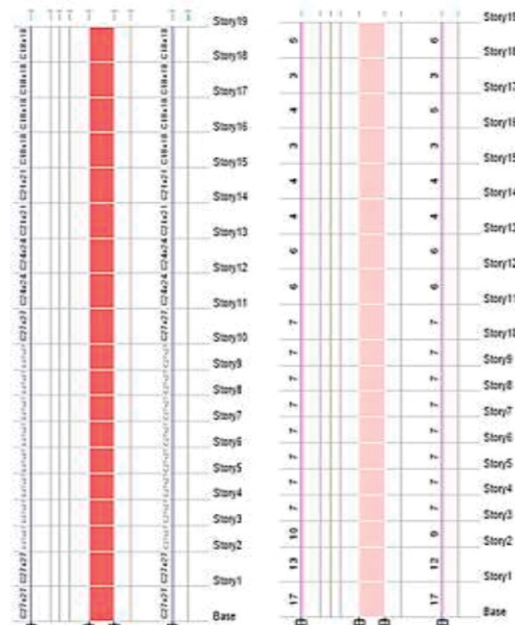
Fig. 21. Column Sizes & Required Area of Longitudinal Steel with L.W.C Floors
